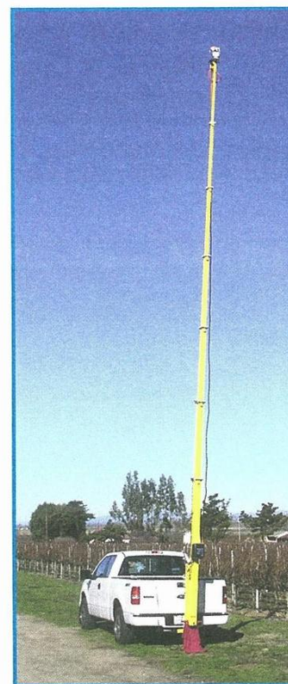
The telescoping mast is extended to 50 feet and is ready for imaging in 10 minutes.
